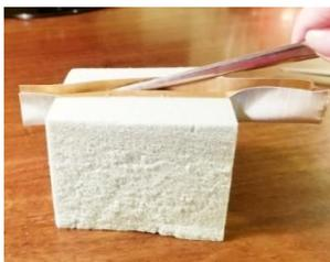
3. Remove block from rim. Cut a 6" piece of duct tape, and fold it in half lengthwise, with the sticky part to the outside. Using a letter opener or butter knife wedge the duct tape into the curved crevice of the foam block, smoothing the tape against the foam to secure. Cut a slit in the excess tape on each side and fold and secure each flap to the sides.
